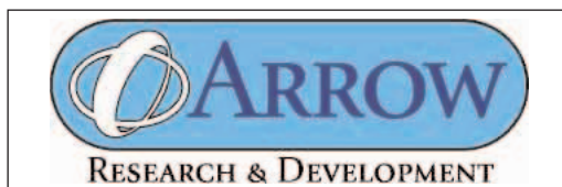
Arrow logo saved incorrectly as a JPEG. (Note the “artifacts”—undesirable miscolored pixels in the white areas.)
